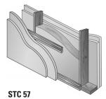
Single 2" x 4" (51 mm x 102 mm) wood studs 24 0C (610 mm), resilient channels: double layer  $^{1}/_{2}$ " (13 mm) Type X gypsum board each side; one thickness  $3\,^{5}/_{8}$ " (92 mm) JM Formaldehydefree thermal/acoustical fiber glass batts.
