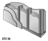
Staggered 2" x 4" (51mm x 102mm) wood studs 24" OC (610 mm): double layer 1/2" (13 mm) Type X gypsum board one side, single layer other side; one thicknesses 3 5/8" (92 mm) JM Formaldehyde-free thermal/acoustical fiber glass batts.
