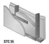
Single 2" x 4" (51 mm x 102 mm) wood studs 24 OC (610 mm), resilient channels: double layer  $^{1}/_{2}$ " (13 mm) Type X gypsum board one side, single layer other side; one thickness  $^{3}/_{8}$ " (92 mm) JM Formaldehyde-free thermal/acoustical fiber glass batts.
