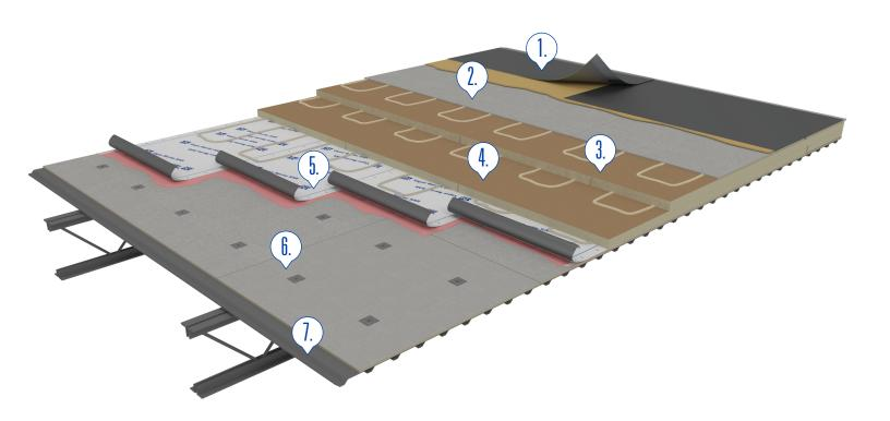
1. JM EPDM NR 90 MIL adhered in JM Membrane Bonding Adhesive (TPO & EPDM). Laps completed with JM 6" EPDM Seam Tape Plus.
