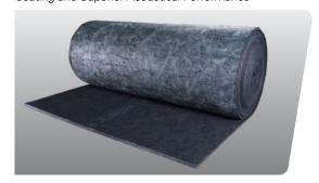
LinacouSTIC® RC-IG insulation is a premium, flexible, fiberglass duct liner madefrom strong glass fibers bonded with a thermosetting resin. The airstream surfaceis protected with JM's exclusive Reinforced Coating System, which combines ourstate of the art Permacote® acrylic coating with a flexible glass mat reinforcementto provide a smooth air stream surface. On the opposite side of the airstream surface, LinacouSTIC RC-IG contains InsulGrip® a non-toxic, water-reactivated adhesive layer.
