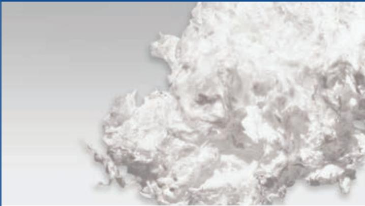
**Q-Fiber®** is an amorphous, exceptionally pure fibrous silica material used as a lightweight, non-crystalline component in high temperature thermal insulations.
