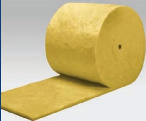
Johns Manville Microlite® B Blanket is a lightweight, flexible, insulating material. This blanket is formed from flame attenuated borosilicate glass fibers and bonded with a thermosetting phenolic resin binder to provide the blanket with strong dimensional stability.
