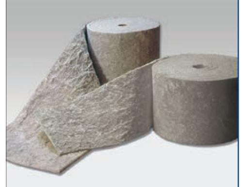
Microlite® AA Premium NR is a lightweight, flexible, thermal and acoustic insulation material designed to provide the ultimate in noise reduction at minimal weight. Microlite AA Premium NR blankets are formed from resin-bonded borosilicate biosoluble glass fibers. An additive is used to provide water repellency to the cured blanket for service in areas where high altitude moisture condensation may occur.
