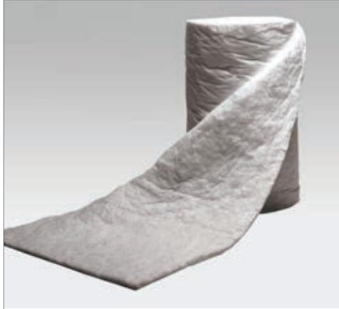
Unbonded Microlite® AA Blanket is a lightweight, binderless insulating blanket designed for thermal and acoustic applications in which intermittent temperatures may reach as high as 1000°F (538°C). This loosely felted, nonresilient blanket is formed from flame attenuated borosilicate glass fibers without binders and oils and is not dimensioned by thickness.
