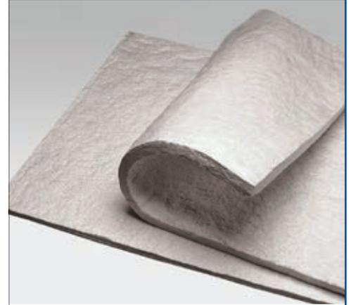
Micro-Fiber® Felt is formed from borosilicate glass fibers using a water deposition process. The result is a clean, flexible, binderless felt with excellent handling qualities.
