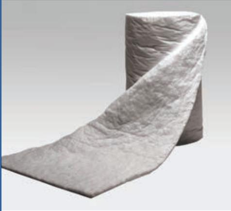
Unbonded Microlite® B Blanket is a lightweight, binderless insulating blanket designed for thermal and acoustic applications in which intermittent temperatures may reach as high as 1000°F (538°C). This loosely felted, nonresilient blanket is formed from flame attenuated borosilicate glass fibers without binders and oils and is not dimensioned by thickness.
