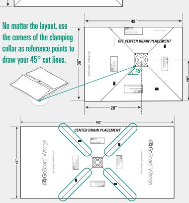
The GoBoard Wedge board seams will match in height, only if you cut them with 45° angles off the corners of the clamping collar.
