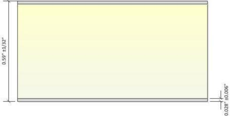
Figure 3: 5/8-in. GoBoard® Thickness Dimensions
