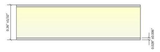
Figure 1: 1/4-in. GoBoard® Thickness Dimensions
