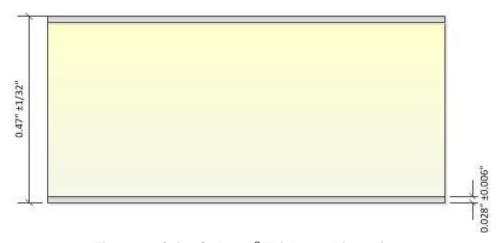
Figure 2: 1/2-in. GoBoard® Thickness Dimensions
